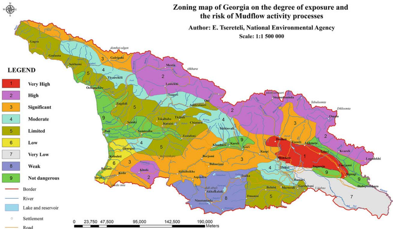
**Fig. 313.2** Zoning map of Georgia on the degree of exposure and the risk of mudflow activity processes
